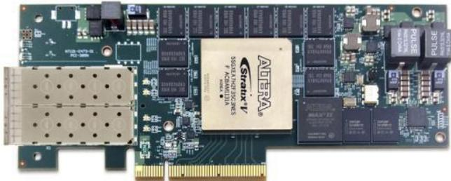
Figure 5. PCIe-385N Stratix V FPGA Accelerator
