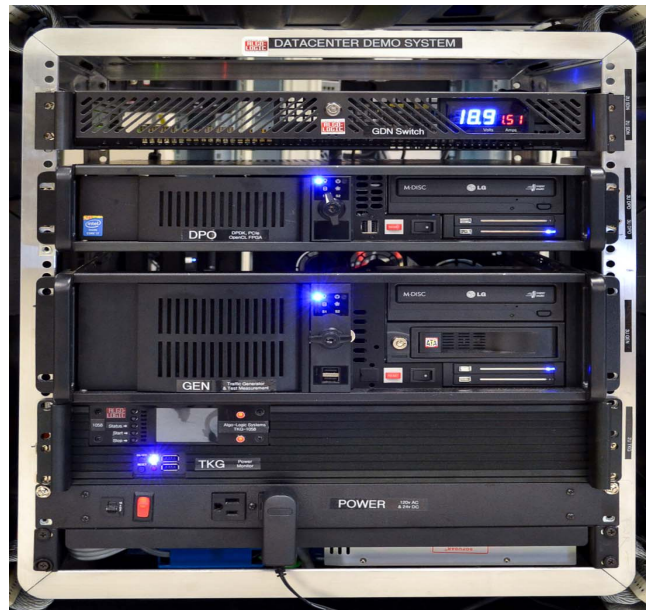
Figure 7: System used to generate traffic, implement KVS, and measure latency, throughput, and power.
