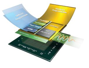
The AMD Zynq<sup>®</sup> UltraScale+<sup>™</sup> RFSoC integrates RF-class A/D and D/A converters into the Zynq<sup>®</sup> FPGA fabric and multi-core ARM processor subsystem, creating a multi-channel data conversion and processing solution on a single chip.
