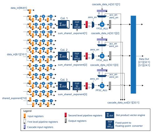
Figure 3. AI Tensor Block architecture
