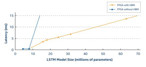
Figure 5. Latency comparison between FPGAs with and without HBM [4]
